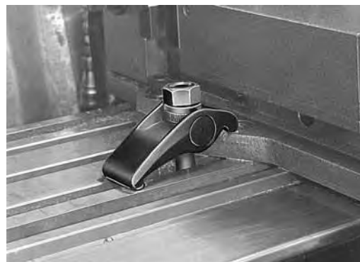
Forged Adjustable Clamp holding one side of a hydraulic vise on a milling machine table.
