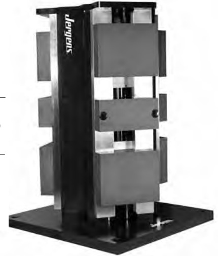
Tri-column design allows up to 240° accessibility
